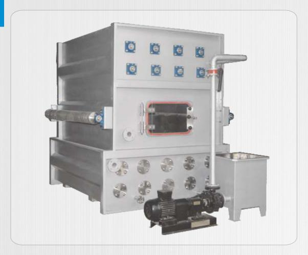
Tank made of AISI 316/304 quality stainless steel.
